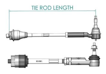
Install the inner tie rod onto the BD Center Link by threading into the link and tightening to spec.
