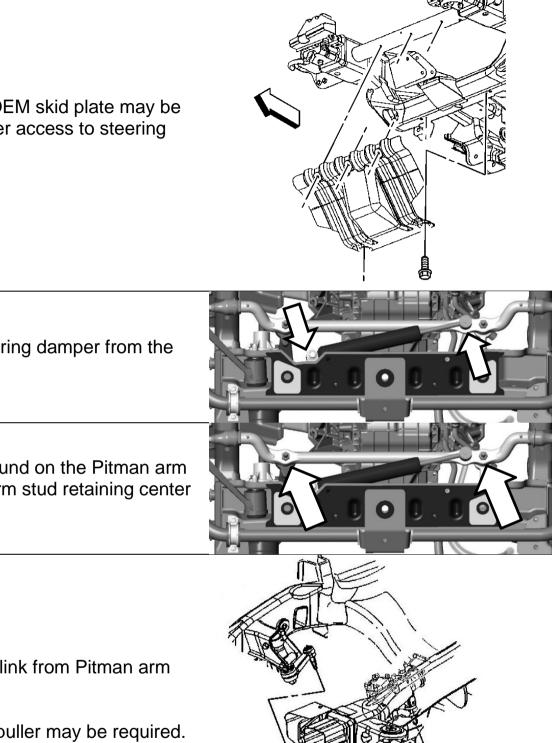
Removing the OEM skid plate may be helpful, for easier access to steering components.
